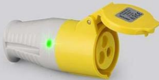
Typ: S1134 with led 16A-4h/100-130V~ 2P+E, IP44 EN60309
